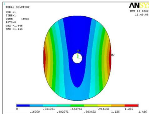
Model of disc bent around pinch belt sort roller
