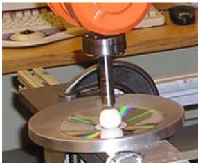
Robotic Hoop Stress fatigue testing.
